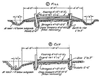
FIGURE 15.-Plank road for motor transportation
