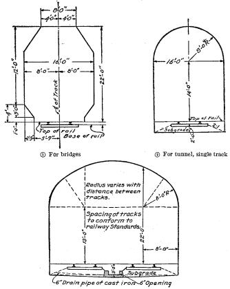
③ For tunnel, double track FIGURE 75.—Standard clearance diagrams for bridges and tunnels
