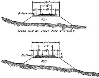
Track laid on wood ties 2-0"C. ro C FIGURE 95.—Section of 60 cm roadbed on embankment
