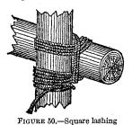
the spar on the side toward which the stress is to come, as it may jam and be difficult to remove. The lashing must be well beaten with handspike or pickhandle to tighten it up. This is called a square lashing.
