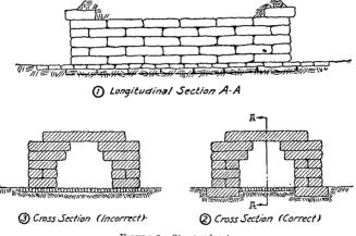
FIGURE 2.-Stone culvert
