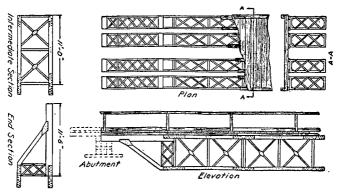
FIGURE 46.—Demountable steel highway bridge
