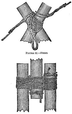
FIGURE 53 .- Lashing for tripod
