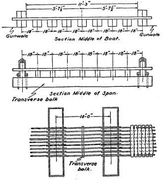
FIGURE 63.-Floor system, heavy bridge equipage, M1924
