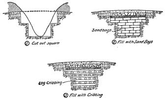
FIGURE 28.-Shell-hole repairs
