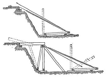
FIGURE 57 .- Erection of trestle bridge
