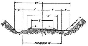
FIGURE 77.-Standard gauge roadbed section in excavation
