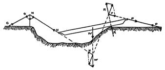
FIGURE 60.-Graphical determination stresses in tackle
