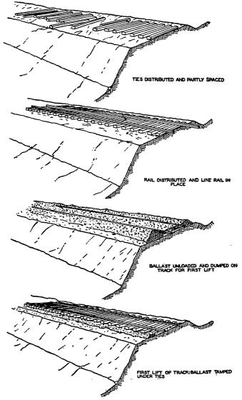
FIGURE 90.-Steps in laying and ballasting tracks
