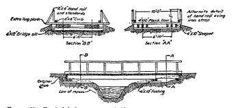
FIGURE 37.—Typical design of stringer bridge showing alternate arrangement of the abutments
