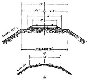
FIGURE 76 .- Standard gauge roadbed section on embankment
