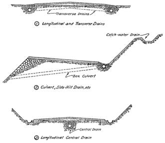
FIGURE 5 .- Foundation drainage (cross sections)
