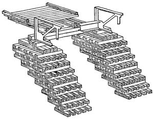
FIGURE 35.-Cribbed abutment
